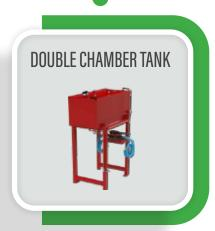
Double-walled fuel tank, with internal stainless steel wall to eliminate the risk of clogged pipes due to oxidation residue, which can guarantee 6 hours operating autonomy at full power. Complete with visual level indicator, low level alarm float connected to the EPRO Control Unit, tank outlet fuel filter and direct support that is autonomously secured to the ground UNI 11292: 2019 6.10.1
