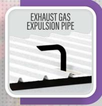
Exhaust gas expulsion pipe of suitable diameter, adequately insulated and protected against accidental contact by means of high temperature ceramic fabric and/or stocking. Exhaust outlet at a height > 2.4 m UNI 11292 6.5.
