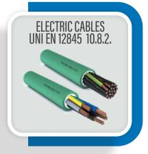
The wiring inside the unit consists of FG16 OM16-0.6/1 kV type cables, compliant with the standard and having a combustion behaviour in conformity with **IEC EN 60332-3-24** and a conductor diameter of at least 2.5 mm<sup>2</sup> of Cu **UNI EN 12845 10.8.2.**
