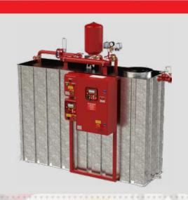
The basic module includes a water storage reserve in hot galvanised steel with a capacity of 2000  $\ell$ , with a main submersible electric pump and a Jockey submersible pump housed inside. All the required hydraulic and electrical accessories to meet the EN 12845 requirements to implement fire-fighting pressurisation units are mounted and connected to the water reserve.
